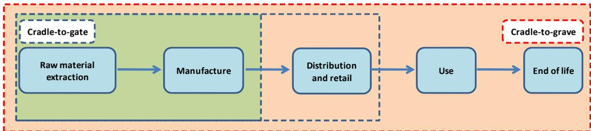
Figure 4. Boundaries determined in cradle-to-gate and cradle-to-grave assessment
