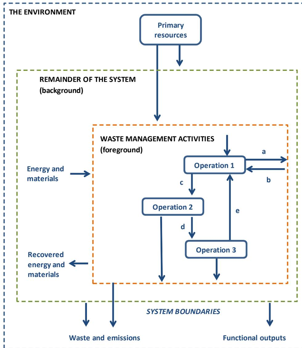
Figure 5. System boundaries in waste management activities (material flows “a” and “b” are open-loop, while “c”, “d” and “e” are closed-loop) (Barton et al., 1996)
